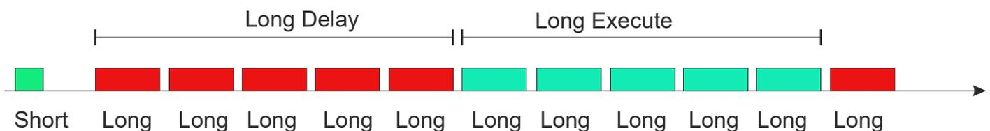
When a short activation of a button is detected, the firmware will detect whether a long activation of the same button in the current mode is being used in the project. If NO, then the short command will be executed right away. If YES, then the firmware will ignore the number of long commands specified in the LongDelay value and carry out the the number of long commands specified in the LongExecute value and then ignore the following long commands.
