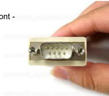
This type of pin-assignment is called DCE (Data Computer Equipment).
